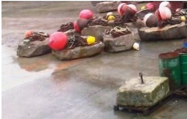
FHC granite 3 tonne blocks, chain and pick up buoys formed the oil boom's moorings.
